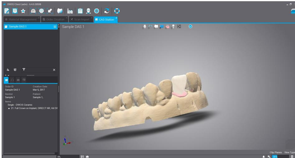
If you want to change the angle of the screw channel, with the right button of the mouse, click on the structure and select “Edit margin line” as in the following image.
