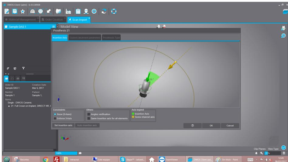
As shown in the image above, the yellow line is the one that allows to move screw channel axis, this axis can freely move in any direction, remember that for titanium bases, it is possible to angle from  $0^{\circ}$  to  $30^{\circ}$  for Regular and wide platforms, and from  $0^{\circ}$  to  $25^{\circ}$  for narrow platforms. This angle value can also be modified when designing the structure.
